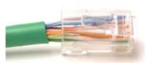
Poorly terminated UTP cable
